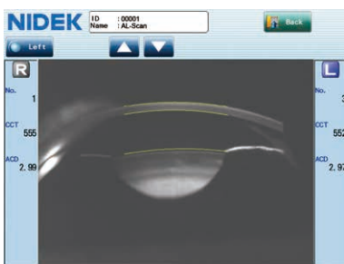
Sectional lens image (Scheimpflug image)
